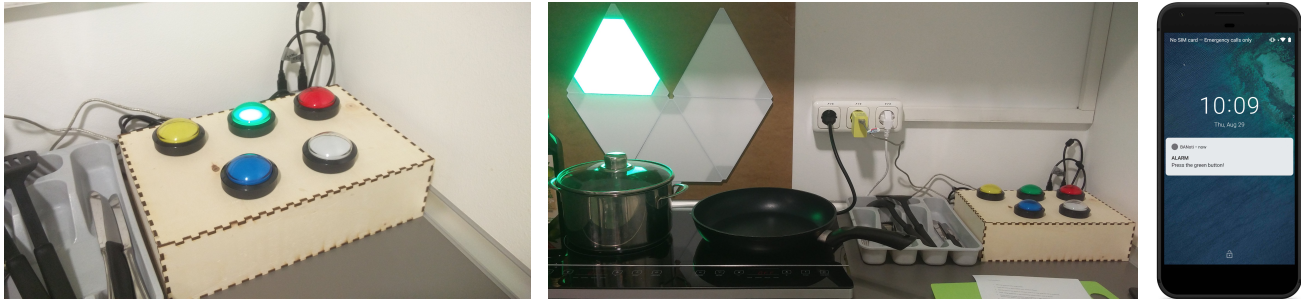
Figure 2: Notification Modalities evaluated in the study. Participants were instructed to either cook with (a) On-Object , (b) On-Environment , or (c) On-Smartphone notifications in a between-subject design.
