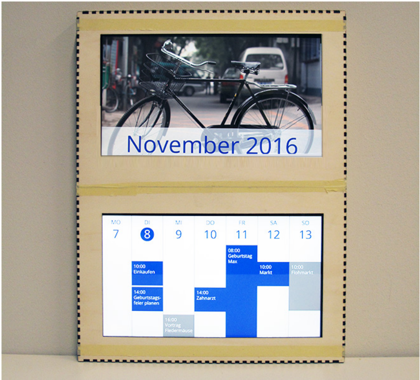
Figure 6.1: The Caloo smart calendar prototype as shown in the pilot study. Event suggestions are entered as entries with gray background.
