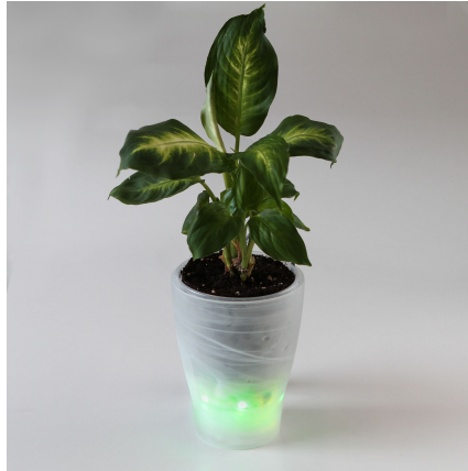
Figure 3.4: The investigated plant pot as a physical prototype representing a plant that has sufficient water
