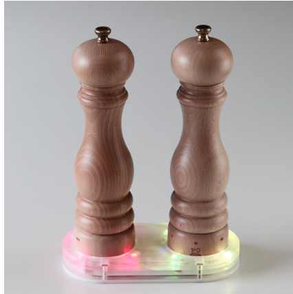
Figure 3.3: The investigated Mill as a physical prototype indicating that the pepper needs to be refilled.
