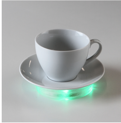
Figure 3.2: The investigated Cup as a physical prototype indicating that the temperature of the coffee is pleasant.
