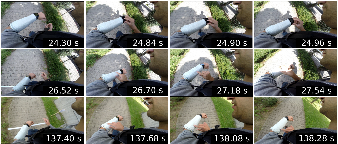
Figure 5. Video recordings of a user performing three different inputs. The user performs input on the smartwatch using touch (top) and two different gestures on the GestureSleeve (middle and bottom).
