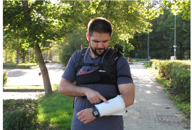
Figure 1. A user wearing the GestureSleeve at the forearm made out of touch-enabled textile. The GestureSleeve is capable of detecting gestures extending the input space of smartwatches.
