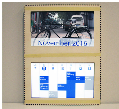
Figure 2. The Caloo smart calendar prototype as shown in the pilot study. Event suggestions are entered as entries with gray background.
