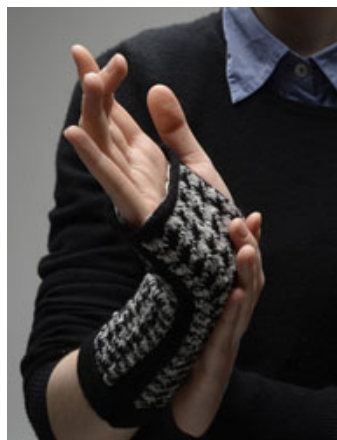
Figure 2: User interacts with a Lorm communication glove.
