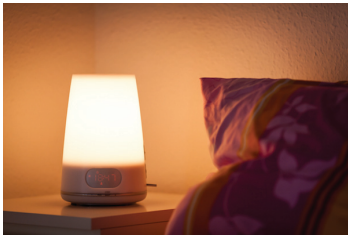
Figure 1: This alarm clock uses ambient light to softly wake up its user. We envision that it could also be used as an helpful output device for other information, e.g., incoming phone calls or reminders.
